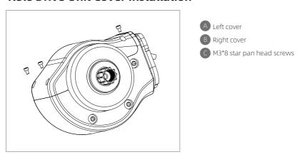
Use a screwdriver (T10) and with three M3\*8 star pan head screws to fasten the motor cover and the interface together, the tightening torque requirement is 0.9-1.0 N.m.
