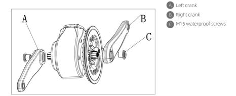
Mount right crank on the right shaft, with internal hex wrench fasten the M15 screws on the shaft-(tigh tening torque is 45-50 N.m). Same way will left crank mount on the shaft (Note: Please guarantee the left and right crank parallel).
